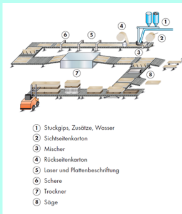
Image 1: Gypsum board manufacturing process; source: Knauf GesmbH
